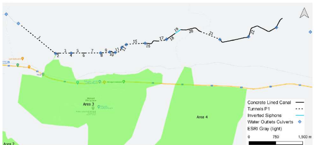
Figure 5: Package 1 - Main Canal Features 14
